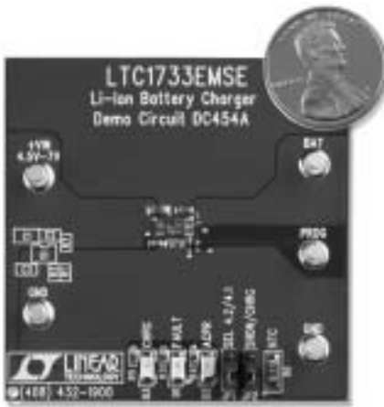
Figure 2. Full featured single cell Li-ion charger
