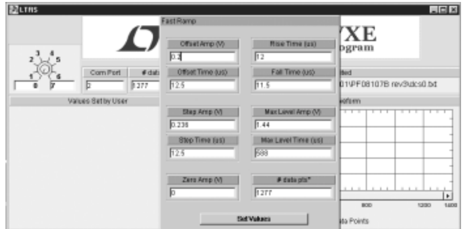
Figure 10. Ramp profile waveform parameter editing window
